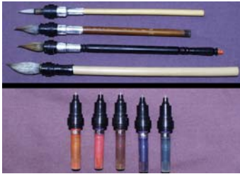
Oriental brushes (above) and ink pens (below) with adapted to fit the plotter drawing arm.
